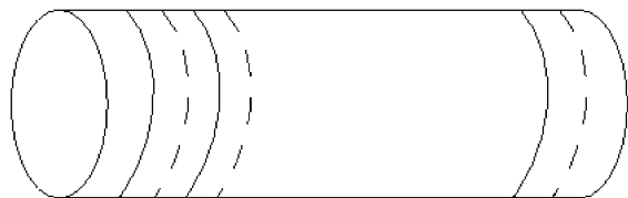
Fig. 1. Drawing of anode configuration of the helical detector. The solid and dashed lines represent two different wires wound about the ceramic core comprising the collecting and non-collecting anodes.
