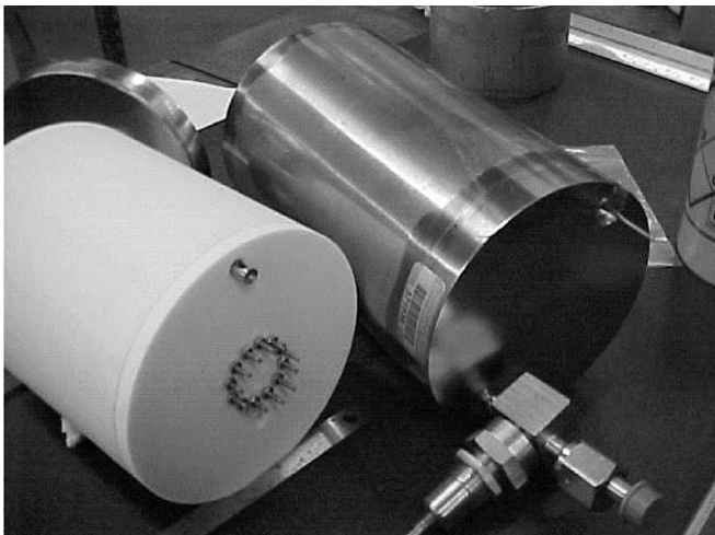
Fig. 7. A view of the detector before final assembly. The white cylinder is the Macor structure that: (i) supports the anodes (protruding from the end); and (ii) supports the cathode, which is a film lining the interior of the Macor shell. The Macor structure is about to be fitted into the pressure vessel from the far end, which will then be welded shut.
