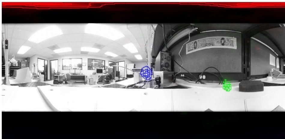
Fig. 4. The spatial deconvolved image from a simultaneous measurement with Cs-137, Na-22, and Co-60 sources, overlaid on an optical panoramic image. The images for energy windows around the primary emission lines of Cs-137, Na-22, and Co-60 are shown in red, green, and blue, respectively.
