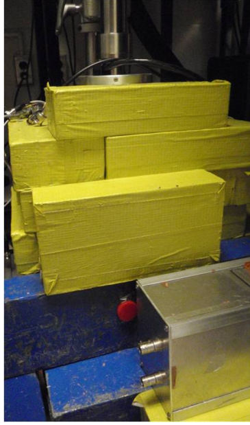
Figure 5.10: Picture of the setup used for measurements of ^{137}\text{Cs} gamma rays that are backscattered in the CdZnTe detector and absorbed in the HPGe detector.
