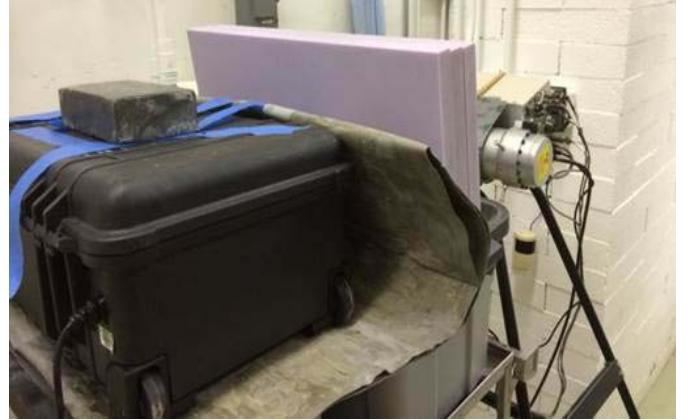
Fig. 12. Experimental apparatus with CdZnTe array inside black Pelican® case, lavender sheets of borated polyethylene, and the neutron generator tube behind. The metallic shielding was used to eliminate bremsstrahlung.
