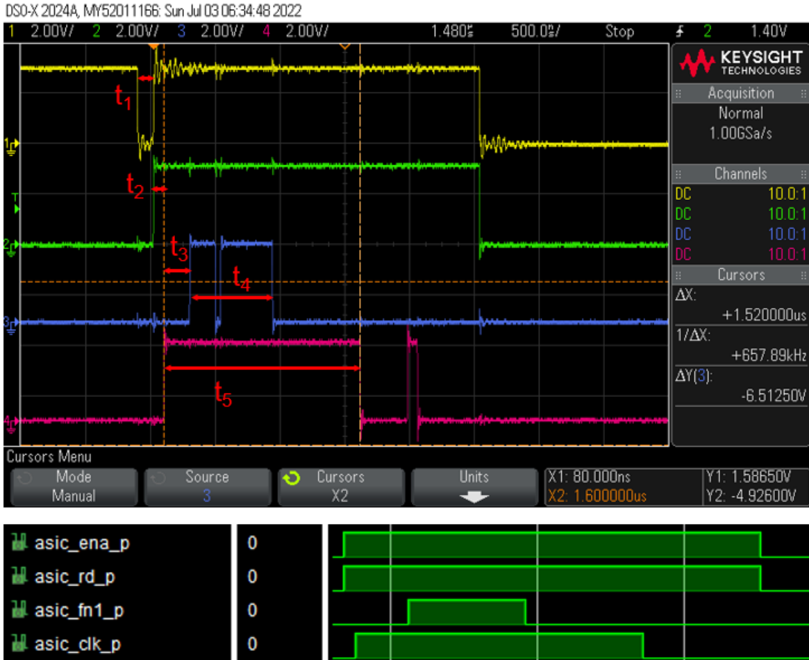
Figure 2.26: Output signals from the on-chip H3DD_Core module at -30^{\circ}\text{C} in response to an ASIC_gReset command sent over SPI. On the bottom is the expected output from behavioral simulation. The measured matches the simulated in broad morphology, but several timings are modified and glitches are present in some of the signals.
