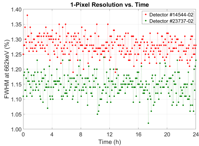
Figure 4.36: The depth-corrected single-pixel energy resolution for Kromek detectors #14544-02 and #23737-02 over a \sim 24 h period at 60°C and -2000V bias.
